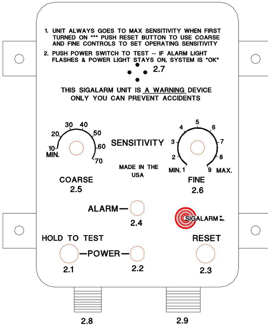
**2.1 HOLD TO TEST BUTTON** - allows the operator to test the entire system by pushing and holding down this button. This button then checks the entire system, if the green power light stays on, external horn sounds, internal buzzer works, and red light flashes the system is fully functional. If any of these are not working contact your supervisor and fix prior to use. If any of these fail there is either a break in the antenna, a jumper pin problem, or there is an internal failure.
