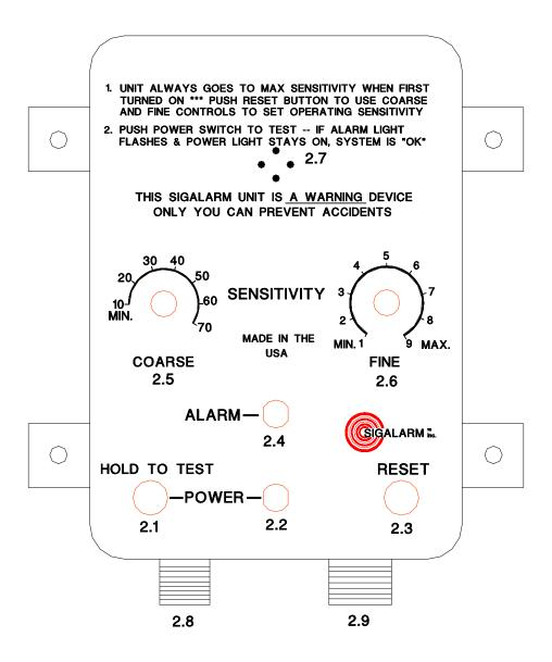
**2.1 HOLD TO TEST BUTTON** - allows the operator to test the entire system by pushing and holding down this button. This then checks the entire system. If the green power light stays on, external horn sounds, internal buzzer works, and red light flashes the system is fully functional. If any of these are not working contact your supervisor and fix prior to use. If any of these fail there is either a break in the antenna, a jumper pin problem, or there is an internal failure.
